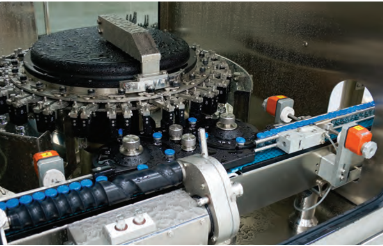
IP69K rated hygienic clamping assemblies make equipment easier to clean and protect against harmful bacteria.
